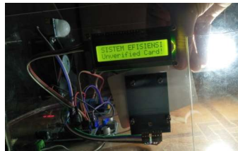
Figure 11. The RFID module detects unregistered cards.
